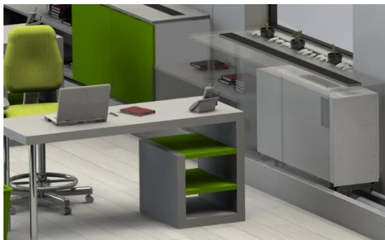
Schematic view from inside the room : the AHPP is installed against the wall close to the window
