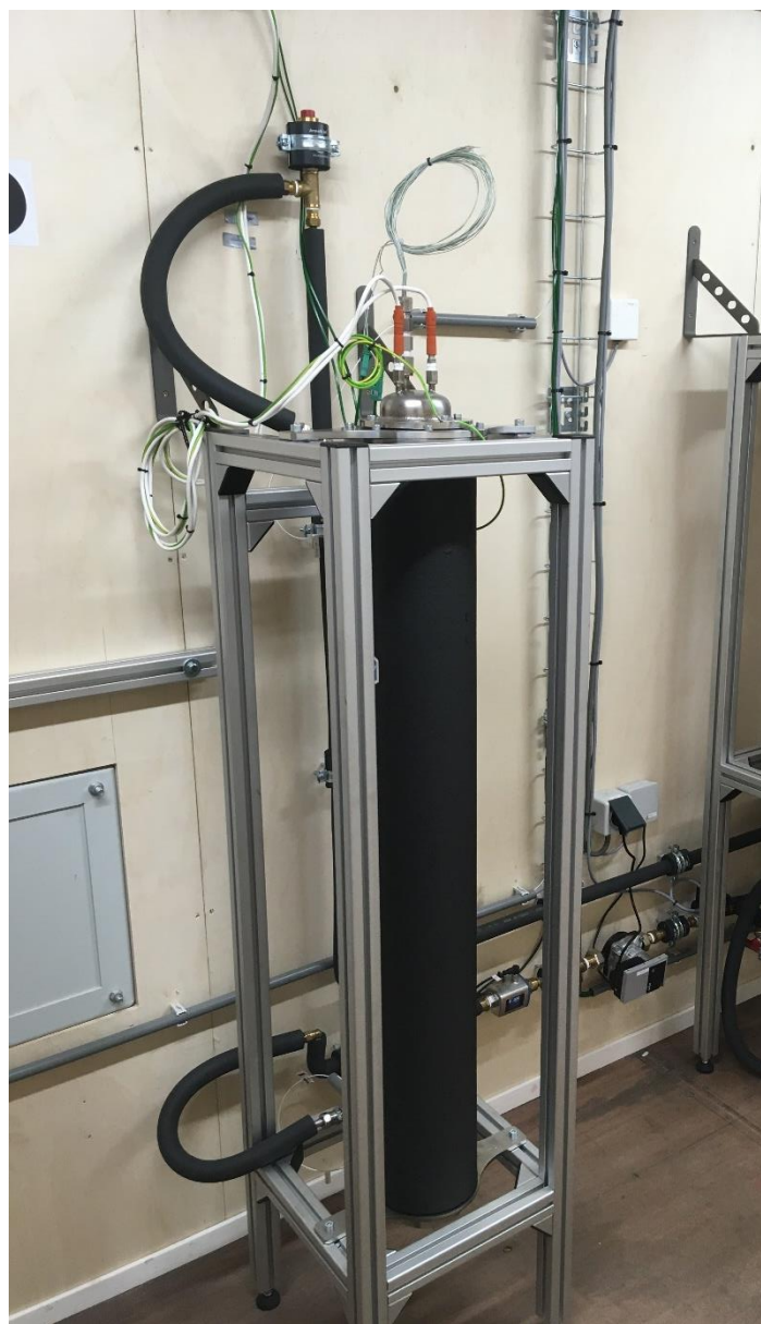
Figure 6: Day 30 of construction, receipt and installation of CLC Emulator Demo Reactor.
