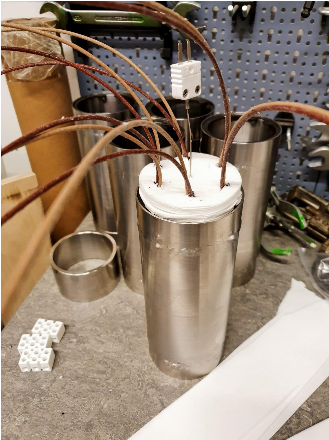
Figure 9: CLC Emulator cartridge fitted with a representative copper mesh and electrical heaters.
