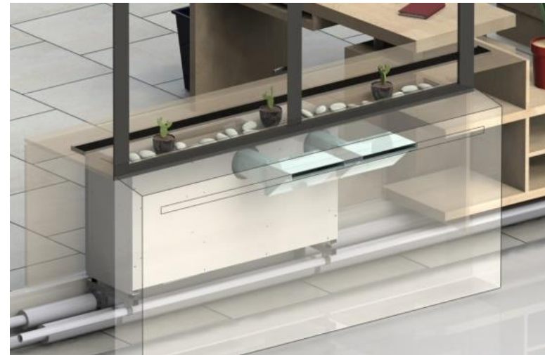
View from outside : 2 ducts integrated in the façade (equivalent diameter 200mm)
